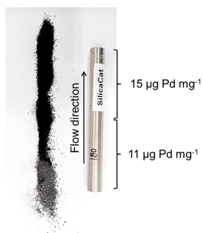
Figure 11. Visual appearance of the content of a used SiliaCat DPP-Pd catalyst cartridge after a continuous-flow Suzuki–Miyaura reaction with the THF/EtOH/H 2 O/K 2 CO 3 system. The Pd content of different fragments of the solid material, as determined by ICPMS analyses, is also incorporated. Degradation of the solid material at the beginning of the reactor is visually observable (gray coloration).
